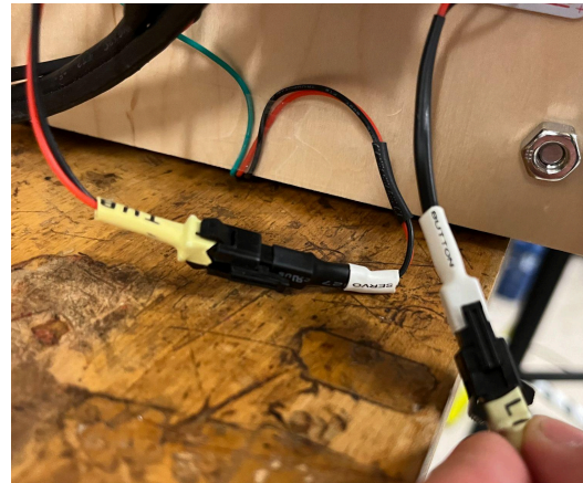
Fig. 1.07 “JST Connectors for Servo and Button”
