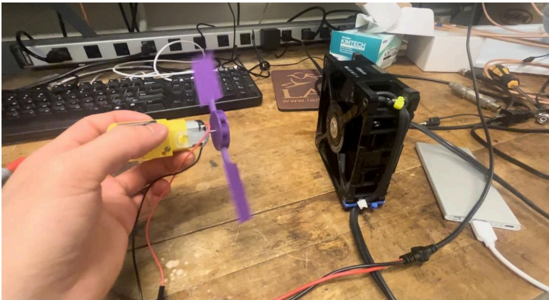
Fig 2.9. “Testing to see if fan will spin the turbine and produce electricity”
